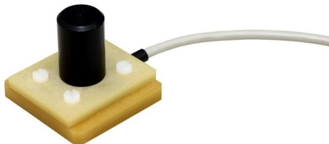
*Fig. 4 : Surface field probe*
