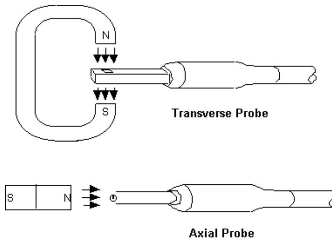
*Fig. 3 : Probe orientation for positive reading*
