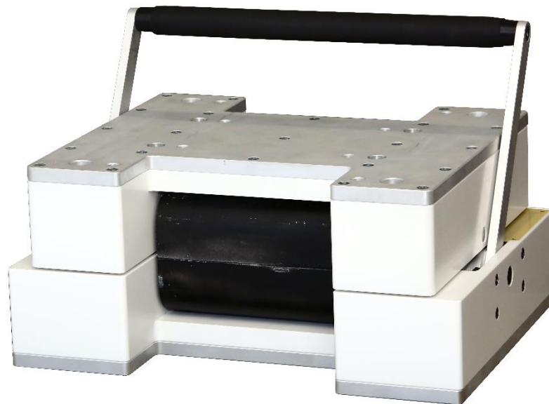
MJC 210 – Small tabletop Single Sheet Tester for the AC hysteresis measurements
